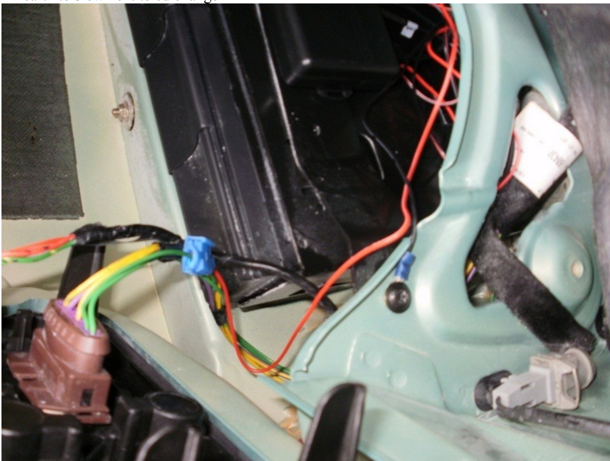
tidy all cables and fix sensor unit in place with double sided tape provided
